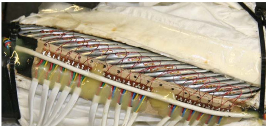
Figure 3: 77 mm rope with strain gauges attached to each of 16 outer wires of one strand.
